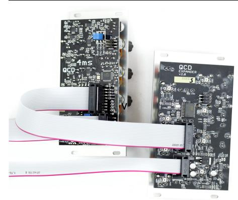
First, remove all the jumpers from the QCD's "EXPANDER" header. Save these jumpers with your QCD box and manual in the bag provided with the QCD. You may wish to use small needle-nose pliers to remove the jumpers if you can't remove them with your fingers.
