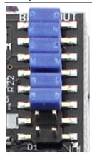
There are six jumpers on the back, and all jumpers must be in place unless the breakout board is in use. The bottom four pins do not get a jumper, they are only used with the SCM Breakout.
